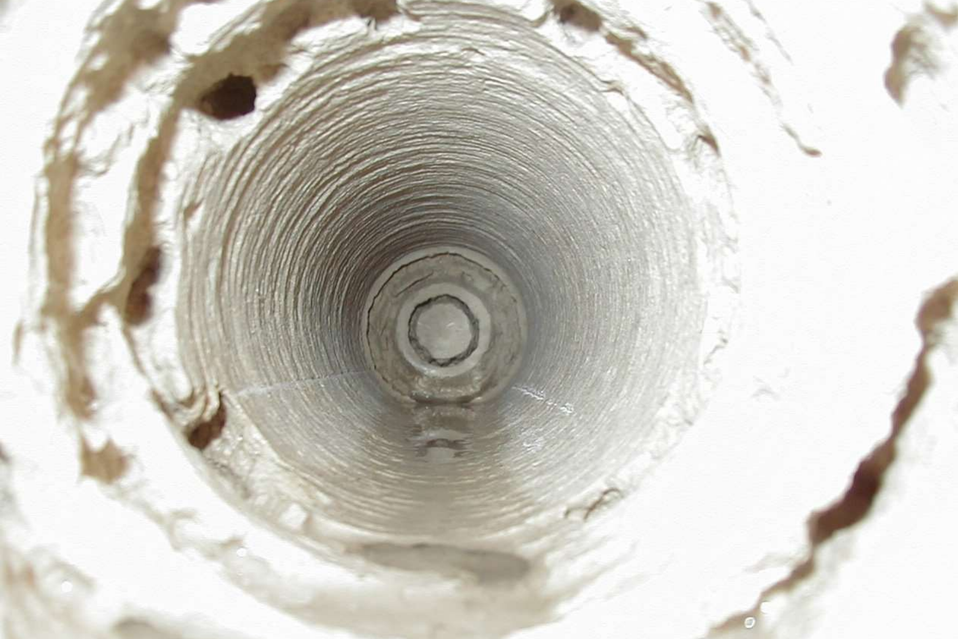
4-3/4 INCH JET DRILLED HOLE – LEUDERS LIMESTONE (MEI)
